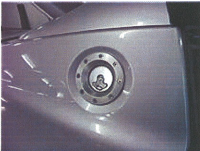
Figure 4: ProAlloyLOTRDC001 Motorsport Fuel Filler Neck fitted to Elise Series 2.
